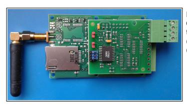
Low dimensions (50.5x77.5mm) and low cost GSM controller. Wireless remote control, temperature monitoring & alarming over dual (900,1800Mhz) or quad-band (850,900,1800,1900Mhz) GSM network.
