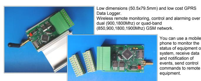
You can use a mobile phone to monitor the status of equipment or system, receive data and notification of events, send control commands to remote equipment.
